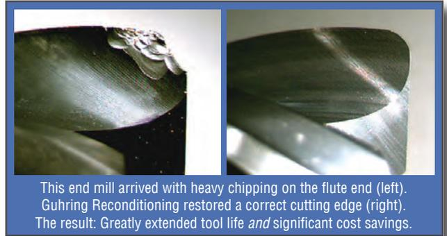
This end mill arrived with heavy chipping on the flute end (left). Guhring Reconditioning restored a correct cutting edge (right). The result: Greatly extended tool life and significant cost savings.
